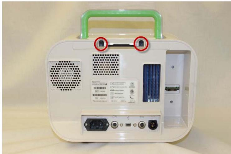
4. Gently pry away the front enclosure to expose the interior of the device.
