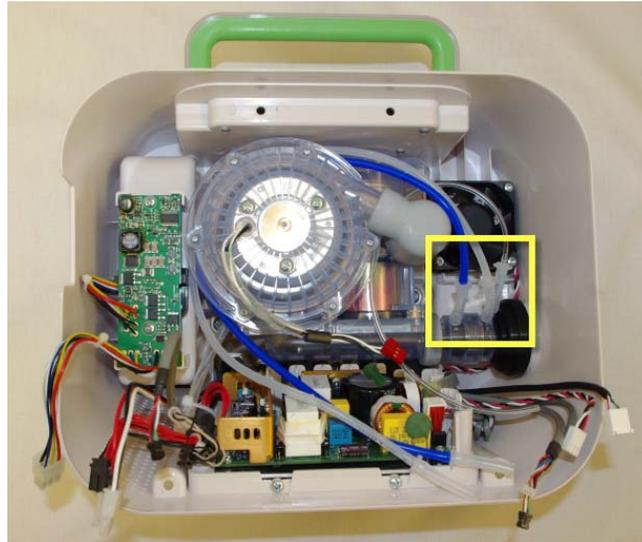
3. Remove the 4 T15 screws securing the Fan to the Rear Enclosure.
