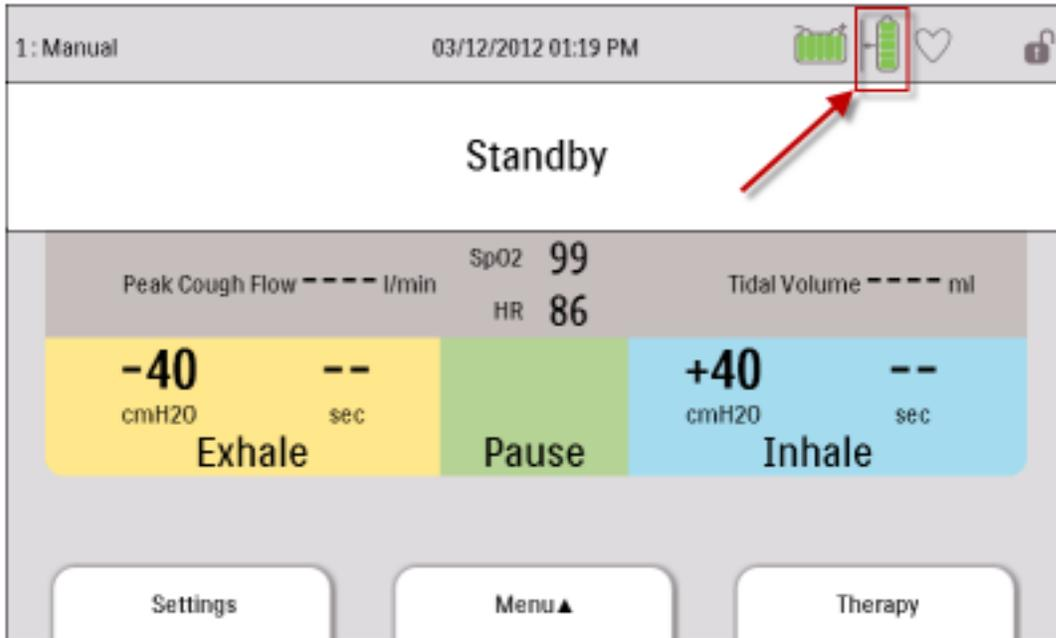
7. Verify that the detachable battery is charging (lightning bolt symbol over the battery). Record the results in the Test Data Sheet.
