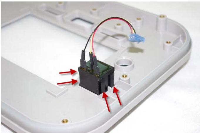
4. Pull the Switch through the front of the Front Enclosure.
