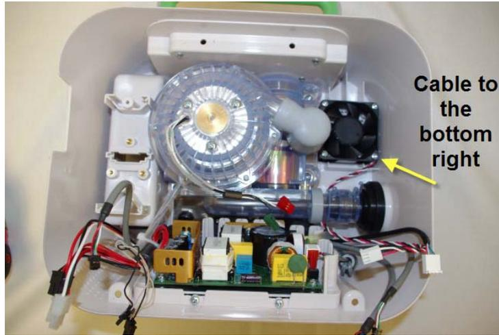
2. Secure the Fan to the enclosure using four T15 screws.
