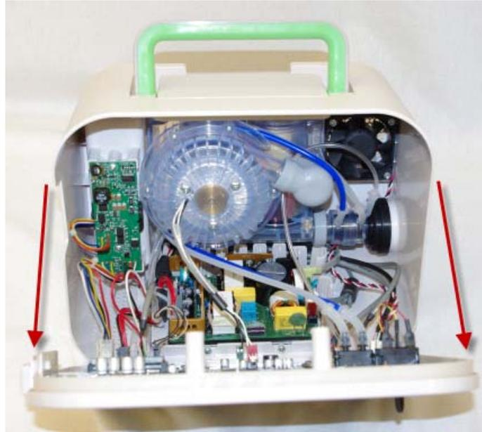
5. Remove the two pieces of tubing from the sensor MT2. The blue tube is connected to the right port and the clear tube is connected to the left port.
