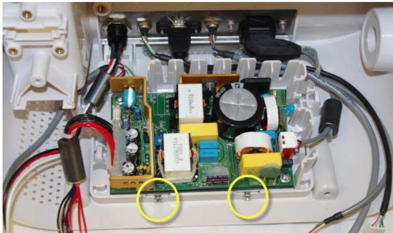
5. Remove the Power Supply PCA from the Rear Enclosure.
