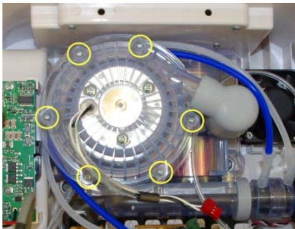
4. Remove the Blower Assembly from the enclosure.
