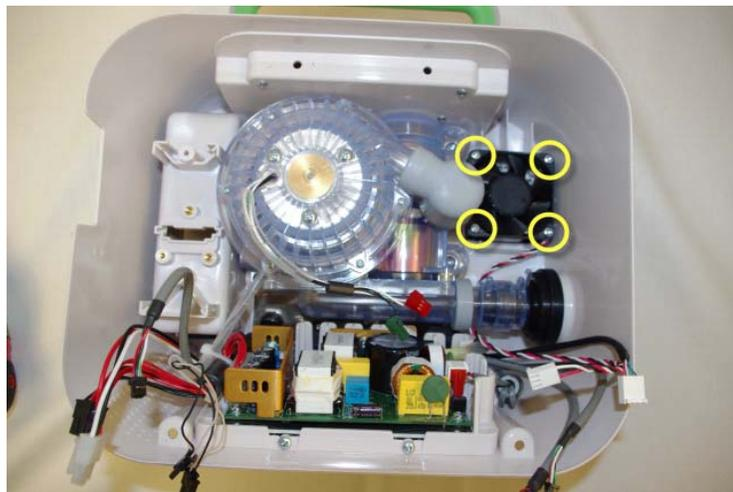
4. Remove the Fan from the Rear Enclosure.
