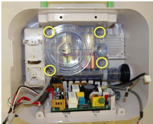
5. Remove the Valve Assembly from the Rear Enclosure.
