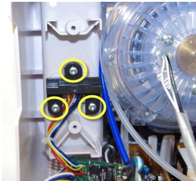
4. Slide the small PCA out of the detachable battery small PCA holder.
