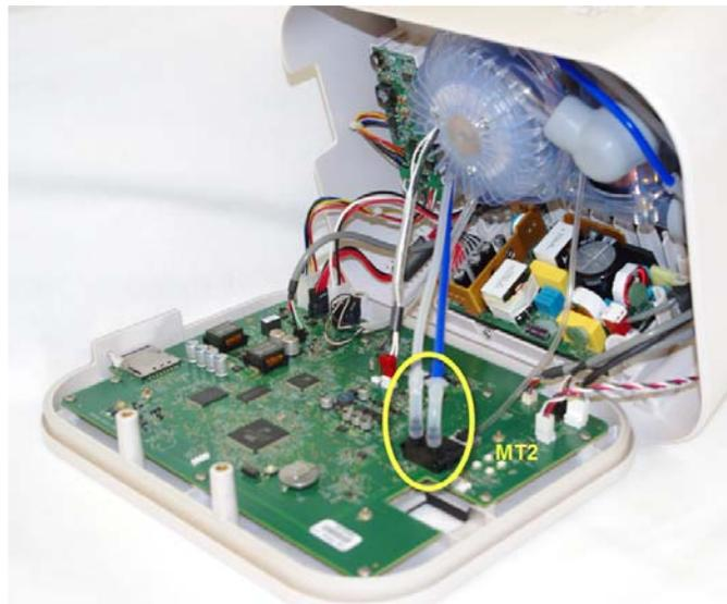
6. Remove the small tube from the top port of the sensor MT5.
