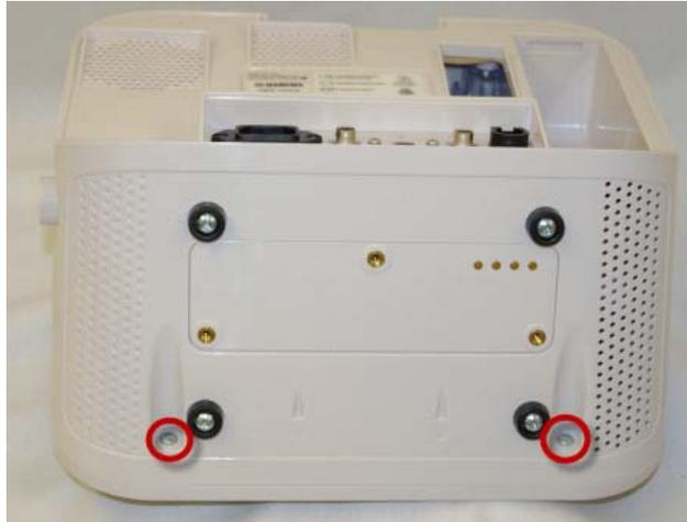
3. Using a T20 Torx bit remove the two screws from behind the handle recess area on the top of the device.
