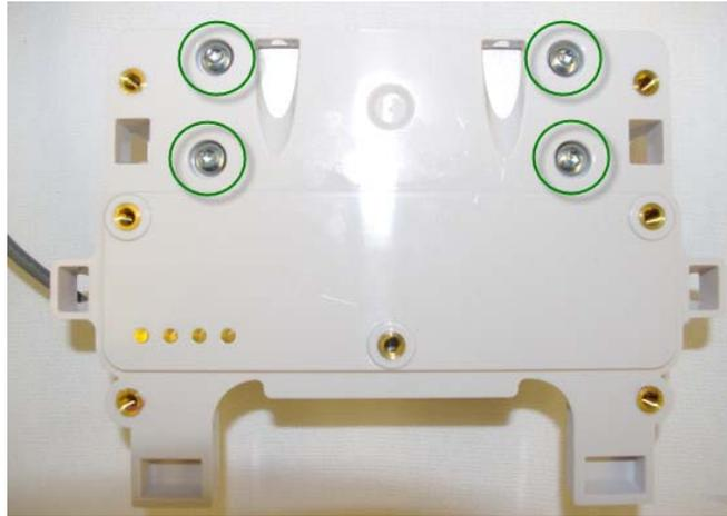
7. Remove the Power Supply PCA.
