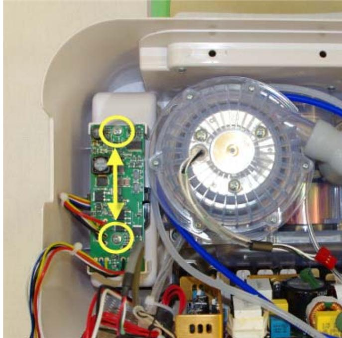
3. Remove the three screws securing the Detachable Battery small PCA Holder to the Rear Enclosure.
